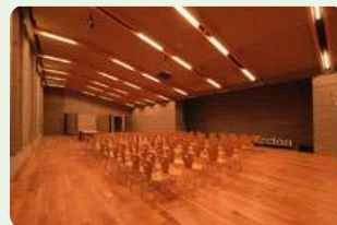
◀ Wood-grain formwork panels removed after structural construction were repurposed as wooden flooring for the first-floor corporate exhibition hall
