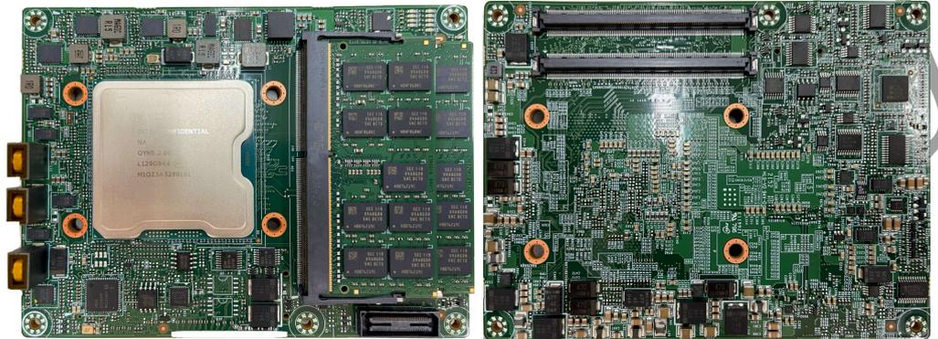
The product is a basic form factor Computer-On-Module (COM) board that is designed to support a wide range of applications primarily in the commercial market segment. It is a Powerful Module in the COM roadmap and is therefore designed to be compatible with the existing System boards as well as FRS customer carrier boards designed to accept other Type 7 basic form factor COM Express module. The COM mezzanine form factor is the “COM Express” standard from PICMG
